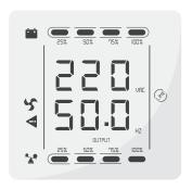
Output: Display the output voltage and output frequency of the UPS. As the following graphic shows, the output voltage is 220V, the output frequency is 50Hz.
