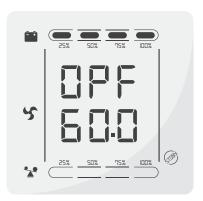
If frequency converter mode is enabled, you may choose the following output frequency:
