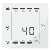
**Temperature:** Display the maximum temperature of the components in the UPS. As the following graphics shows, the maximum temperature is 40°C.
