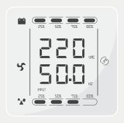
**Input:** Display the voltage and frequency of the input. As the following graphics shows, the input voltage is 220V, input frequency is 50Hz.
