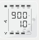
**Load:** Display the numerical value of the active power (WATT) and apparent power (VA) of the load. For example, as the following graphics shows, the WATT of the load is 800W, VA is 1.0KVA (when disconnect loads, it is a normal phenomenon to show a small numerical value of WATT and VA).
